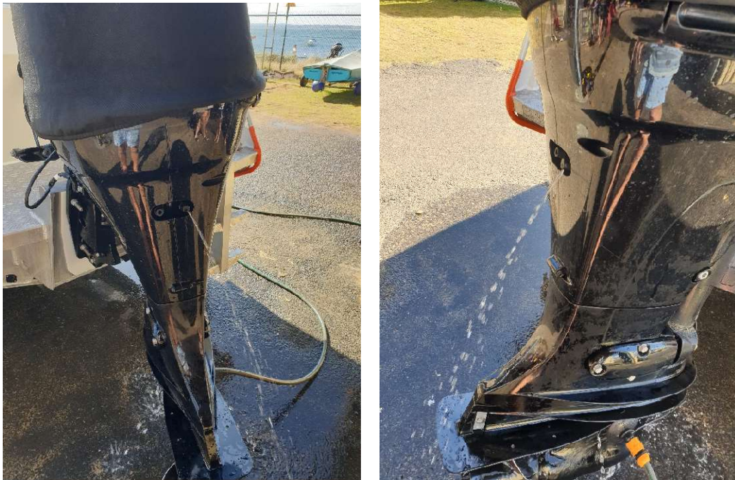
Figure 6 – Ensure water exits motor as shown
