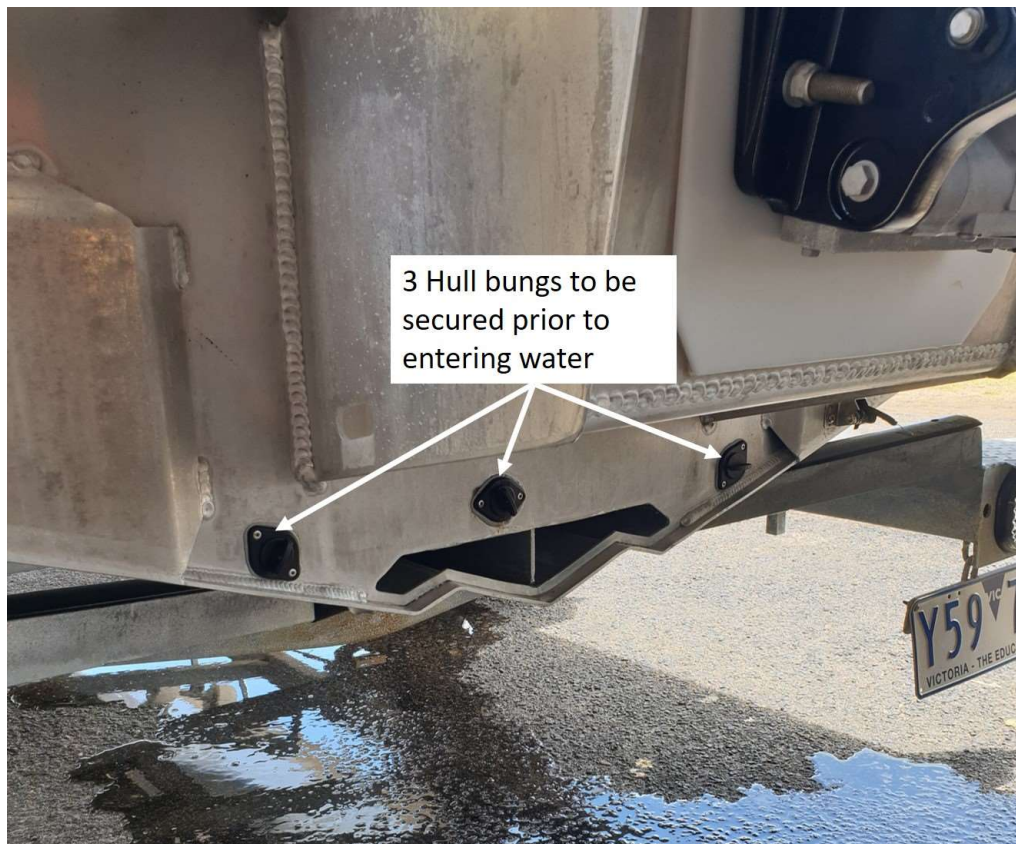
Figure 4 – Three hull bungs must be inserted
